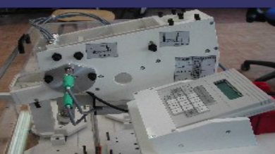
Overview of the machine BBA 0306 with the oval conveyer, without hoisting unit (elevator) and with the counter in the middle
